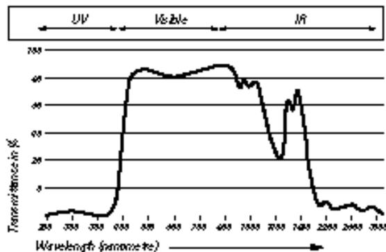
**Clear Lexan solid sheet** Clear Lexan solid sheet offers excellent clarity almost approaching that of glass, with light transmission values of 75 – 87%, depending upon the thickness of sheet. However, for buildings in hot climates or with south facing aspects, Lexan solid sheet is available in translucent grades of bronze, grey and opal white.
